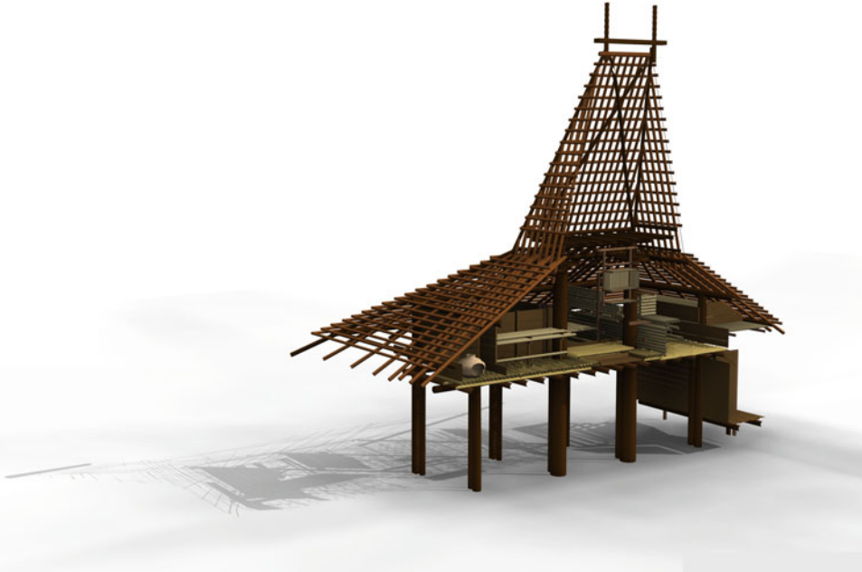
Architecture in Sumba, Fig. 3 3D section of an uma mbatangu , showing different types of posts supporting floor, roof and attic, the towering roof structure, and the design of the interior space (©R. Humenberger & author)
