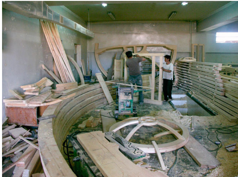
Architecture: Nomadic Architecture of Inner Asia, Fig. 30 Ger manufacture in Ulan Bataar
