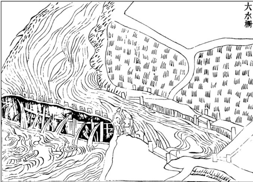
Agriculture in China, Fig. 9 A large sluice across a river, with irrigation channels leading off into padi fields (Nongshu 19/2a–b)
