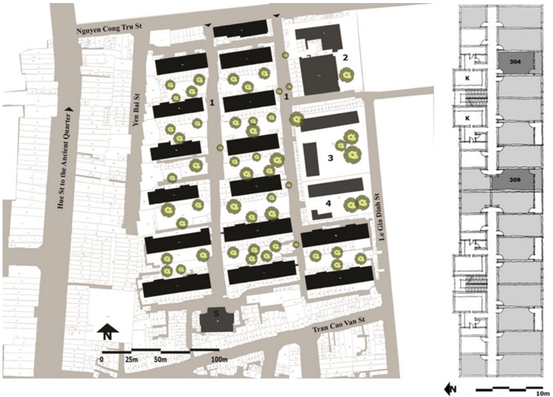
Architecture in Hanoi, Fig. 8 Plan of KTT Nguyen Cong Tru and a typical floor plan of an apartment block
